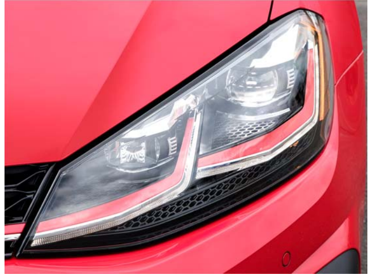
SE & Autobahn have LED headlights w/ Adaptive Front-lighting System (AFS) & LED fog lights w/ low-speed cornering lights
